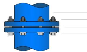
Flanged Component Nuts & Washers Gasket Bolts & Washers
